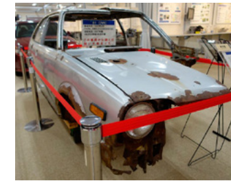
Rust on the body of a Honda Civic made in 1981
